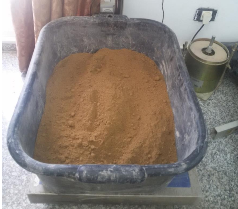
Figure (A.3): Milled clay with water content 8%.
