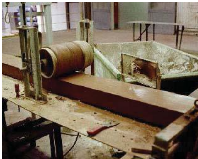
Figure ( 2.9): Brick textures are applied by passing under a roller after extrusion (Brick Industry Association TNT9, 2006).
