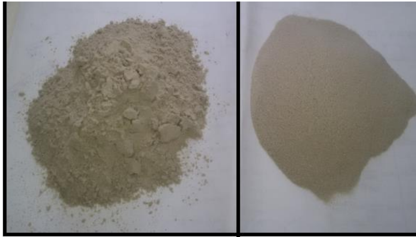
Figure (3.5): Different waste glass particle size (150 \mu\text{m} and 600 \mu\text{m} ).
