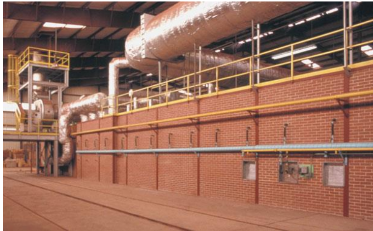
Figure (2.7): A typical tunnel kiln (Mehta et al., 2003).
