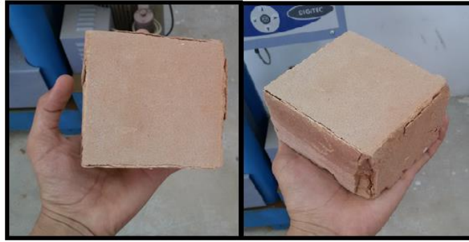
Figure (4.9): Fired clay brick after failure in compression.
