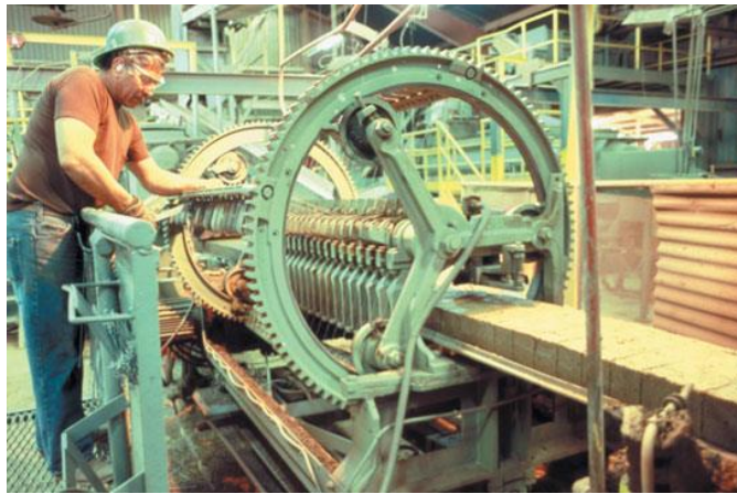
Figure (2.5): Wire cutter cuts the wet clay column into several bricks (Mehta et al., 2003).
