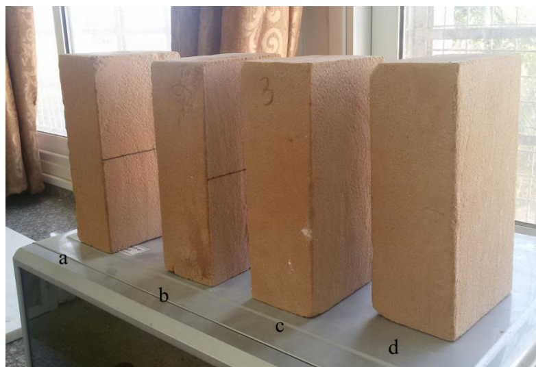
Figure (A.12): Clay bricks fired at 1000C: (a) 0% glass, (b) 10% glass, c) 20% glass, d) 30% glass.
