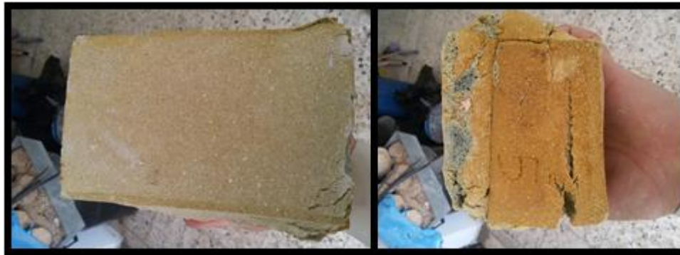
Figure (4.2): Negative firing shrinkage fired clay brick with 40% waste glass and firing at 1100°C.
