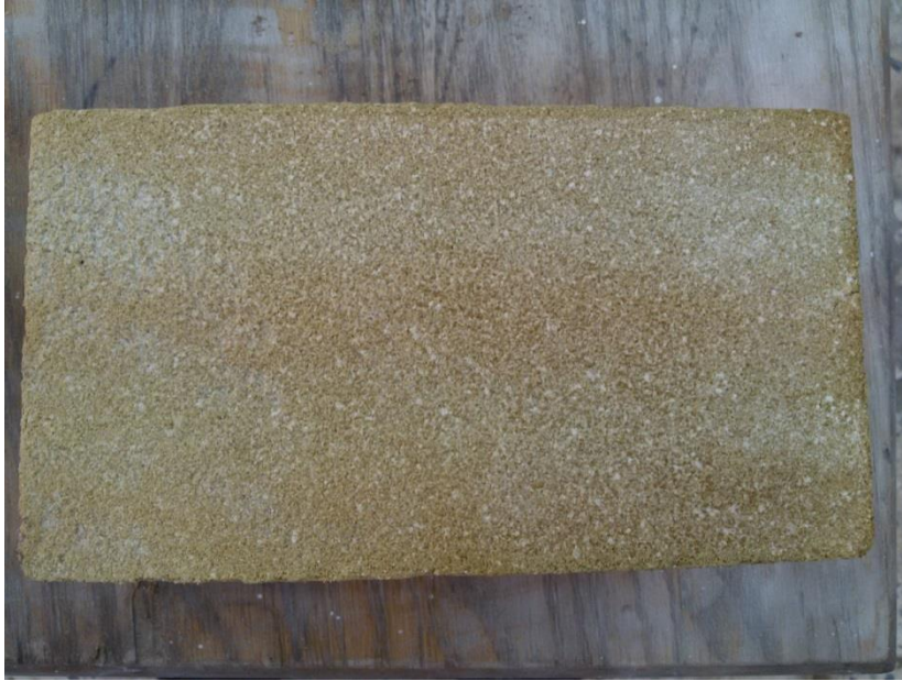
Figure (A.13): Fired clay Brick with 20% waste glass content.
