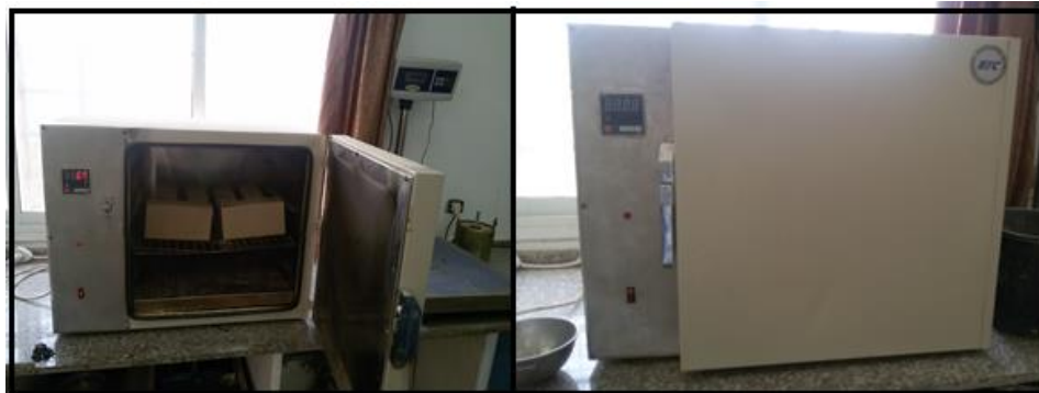
Figure (3.11): Drying brick samples in an oven.
