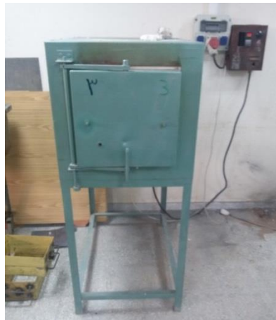
Figure (3.12): Firing brick sample in electrical furnace.
