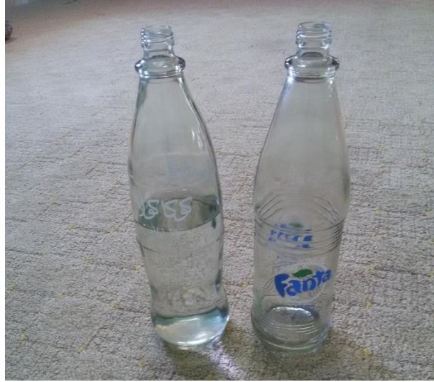
Figure (2.11): Soda-Lime-Silica glass.
